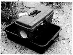
This trap attracts mosquitoes that are looking to lay eggs in stagnant water. There is a fan and collection chamber in the tool box portion of the trap to suck the mosquitoes up and keep them for identification and testing. These represent the majority of the traps we set, as they primarily collect the kinds of mosquitoes that spread West Nile. These traps are generally set in the afternoon and will be retrieved the following morning.
