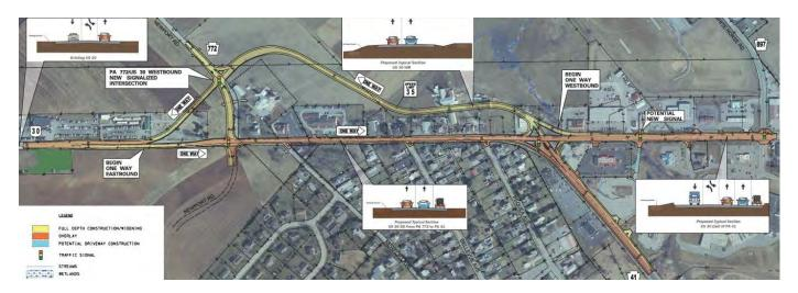
The current design proposal involves creating a one-way loop along Route 30 between Routes 41 and 772. Westbound traffic would travel along a newly constructed road immediately to the north of the current Route 30 alignment. Eastbound traffic would continue to operate on the existing alignment. Signal improvements and roadway widening would occur east of Route 41 to Route 897.
